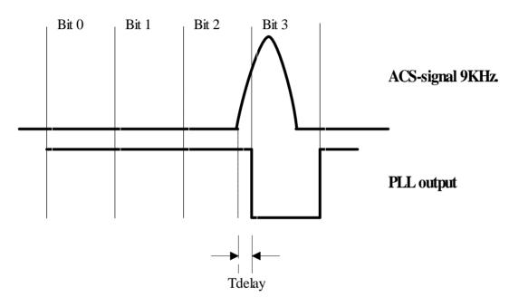
$T_{delay}$  is the delay time from 9 KHz. Presented on input of PLL until valid output. The negative pulse of the PLL is used as the overall trigger for the internal timer in the software UART.
